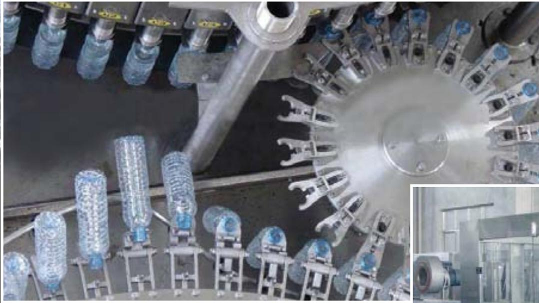
**D**uring the filling process, every bottle is washed using purified ozone water to guarantee 100% sanitation.
