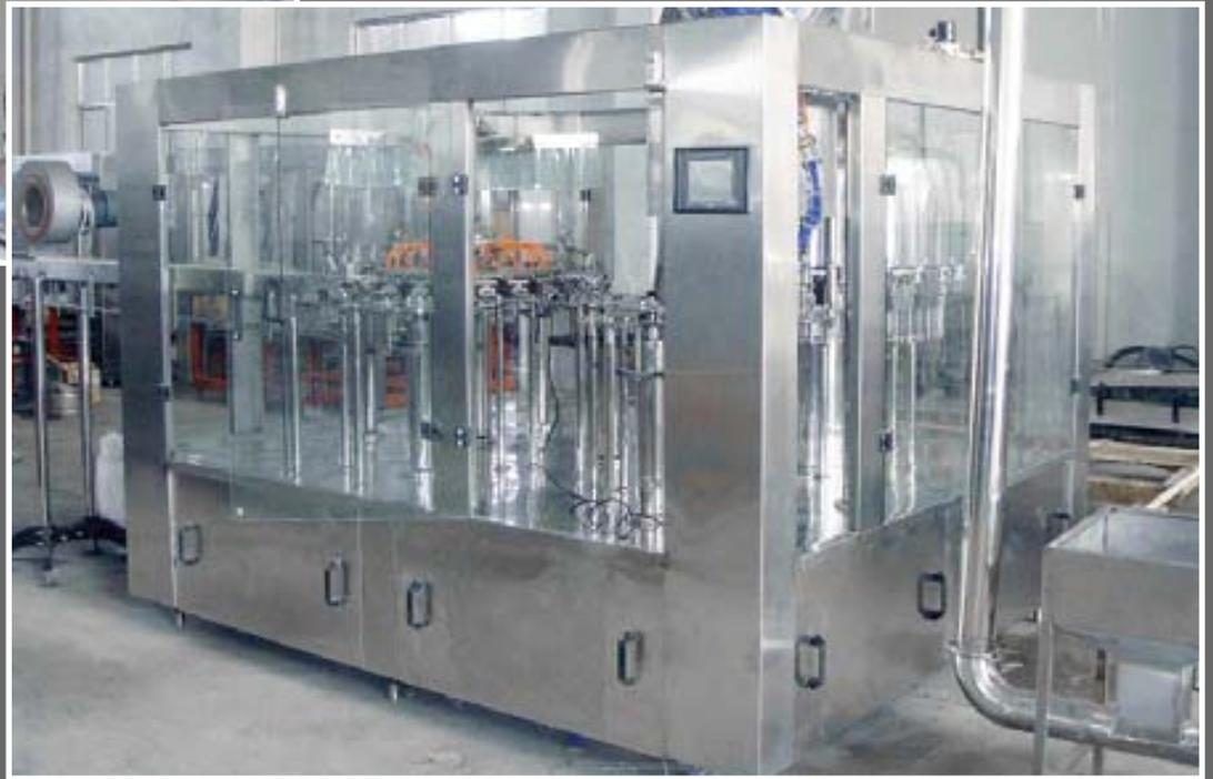
**T**he heart of our bottle production is our unique 3-in-1 filling machine producing more than 9000 BPH in a sterilized environment.
